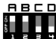
Primary output starts closed. When triggered the output will open until reset.
