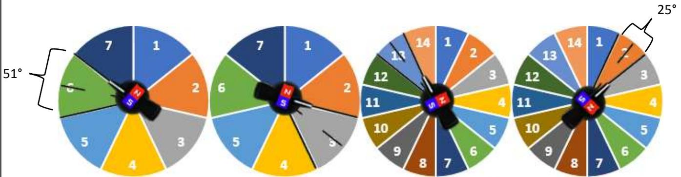
Next adjust the prop pieces to their desired outer limit. Set the FX51-D to
