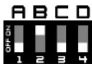
The low threshold configuration triggers at about  $\pm 20\%$  of the detected magnetic field strength.
