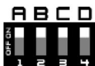
Toggles LED output in case the LEDs are visible through the prop. Keep the switch set to this configuration to prevent accidental mode changes if SET is inadvertently pressed.
