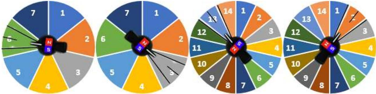
If a custom threshold is desired, follow the steps in **Rotational Learning (Default Radius)**. This will initially set a center point with a 15° radius.
