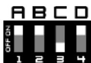
Primary output starts open. When triggered the output will close until reset.
