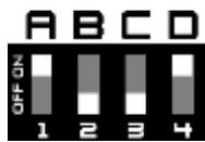
The primary output is closed when triggered, otherwise open.
